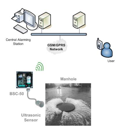
Infinite BSC-50-E is a battery powered RTU/Data logger designed specifically for remote monitoring and alarming. A BSC-50-E unit equipped with an ultrasonic sensor is ideal for open channel flow monitoring featuring advanced relay alarming. Using proven ultrasonic echo ranging technology it is possible to monitor wastewater of any consistency up to 4 m in depth. Achievable resolution is 0.1 % with accuracy
